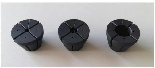
Cuvette holders for cylindrical cuvettes with outer diameter of 5.0mm, 10mm and 20mm.
